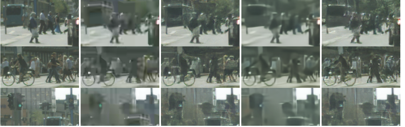
Fig. 2. Effects of compression and restoration (from left to right): captured image, compressed (BPG), restored (BPG), compressed (MSH), restored (MSH). The brightness of the image crops have been slightly enhanced to improve visibility.
