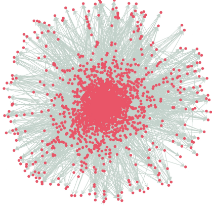
Figure 2: Flight-connection graph of a small \mathcal{L}\mathcal{P} for a CPOP, covering 3202 flight nodes using 21,564 edges in 7991 pairings
