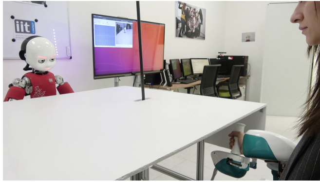
Fig. 1. Left Panel: the setup of the experimental room for the iCub group . The iCub robot (A) is standing in front of the participant (B), who is sitting next to the Wristbot (D). The pendulum is between them (C), while the experimenter (E) is hidden behind a black curtain. For the Control group , the set-up was the same except for the iCub robot that was hidden behind another black curtain. Right Panel: The robot gazing with a focused expression at the participant, who is trying to balance the pendulum using the Wristbot.
