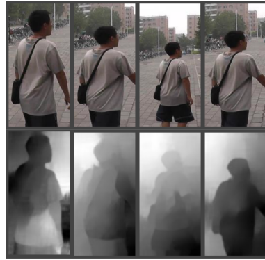
Figure 2. Example of a sequence of bounding boxes images from the MARS dataset (top row), and its corresponding dense optical flow map (bottom row). The common saliency in the sequence can be observed from the optical flow map.
