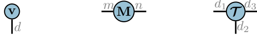
Figure 1: Tensor network representation of a vector \mathbf{v} \in \mathbb{R}^d , a matrix \mathbf{M} \in \mathbb{R}^{m \times n} and a tensor \mathcal{T} \in \mathbb{R}^{d_1 \times d_2 \times d_3} .
