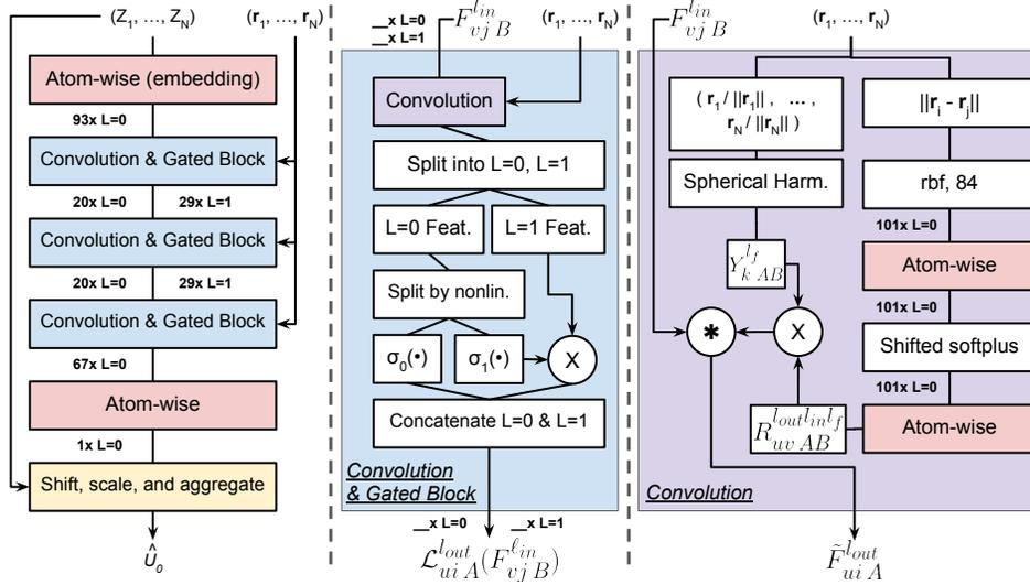
Figure 1: Illustration of L1Net with the architecture on the left, the convolution & gated block in the center, and the convolution on the right. The scalar activation function  $\sigma_0(\cdot) = \text{Softplus}(\cdot)$ , while the gated activation function  $\sigma_1(\cdot) = \text{Sigmoid}(x)$ . The notation “ $T \times L = D$ ” implies that this connection contains a multiplicity  $T$  of features with degree  $D$ . The target output  $\hat{U}_0$  is shown as an example.
