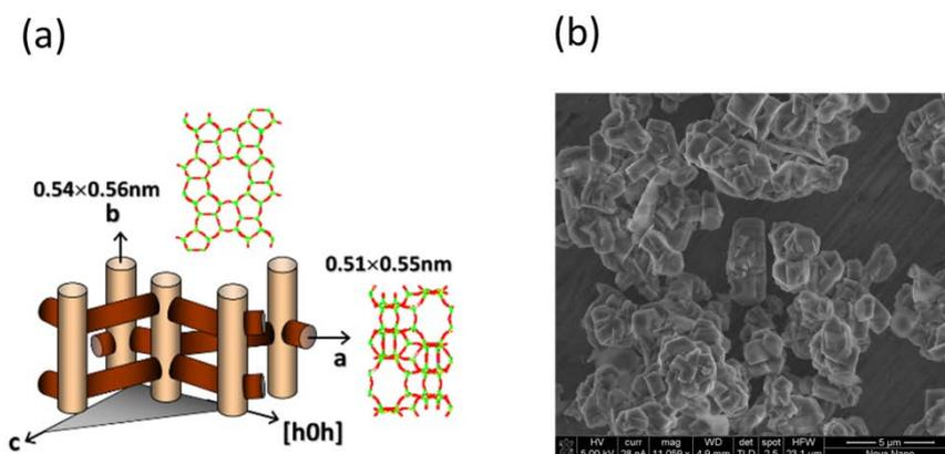
Figure 1. (a) A cartoon picture of ZSM-5's skeletal pore structure. (b) A SEM image of the ZSM-5's crystals. Each crystal is about 2 to 3 microns across.
