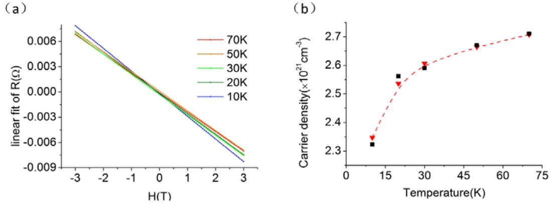
**Figure 5. (a) The temperature dependence of Hall resistance for nano-carbon@ZSM-5. (b) A comparison between the electronic charge carrier density obtained from by the Hall measurements (black symbols) and that obtained from fitting of the longitudinal differential resistance peak values vs. temperature in nano-carbon@ZSM-5 (red symbols). The red dashed curve is to guide the eye.**
