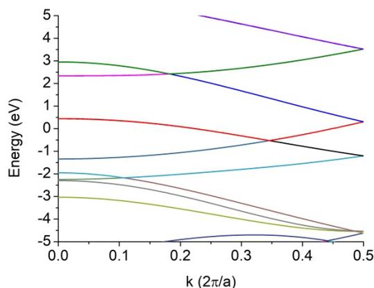
**Figure S1. Calculated band structure of (3,0) CNT. In the spectrum the energy=0 denotes the Fermi level. It is seen that there are a total of 3 bands crossing the Fermi level, which may induce electron-phonon coupling.**
