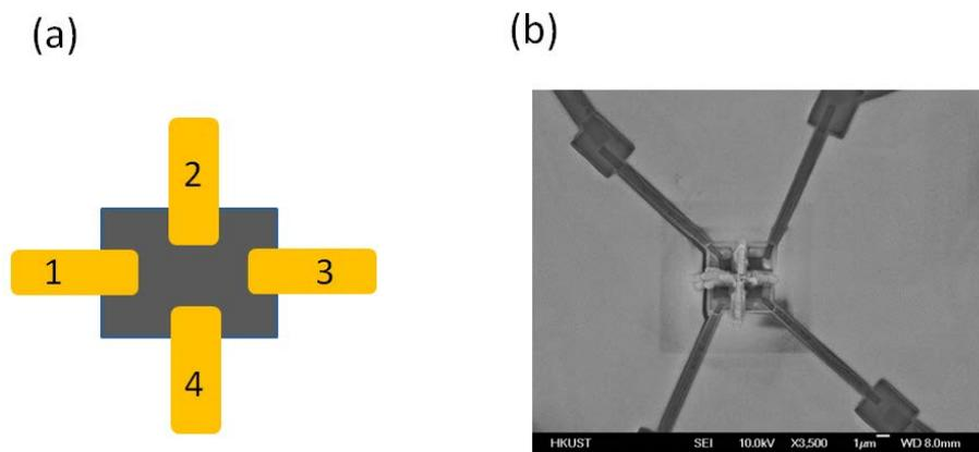
**Figure 2. Device for transport measurement. (a) Schematic illustration of the four-terminal geometry. (b) A SEM image of the four-terminal device for electrical measurement. The size of the nanocarbon@ZSM-5 sample is about 4 microns.**
