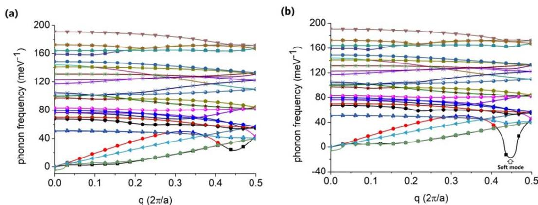
**Figure S2 (a) The phonon spectrum under a smearing broadening of 0.1 eV. (b) The phonon spectrum under a smearing broadening of 0.05 eV. We find that at the 0.05 eV broadening, which corresponds to 273 K, an imaginary phonon frequency occurs, indicating a Peierls transition at this temperature.**
