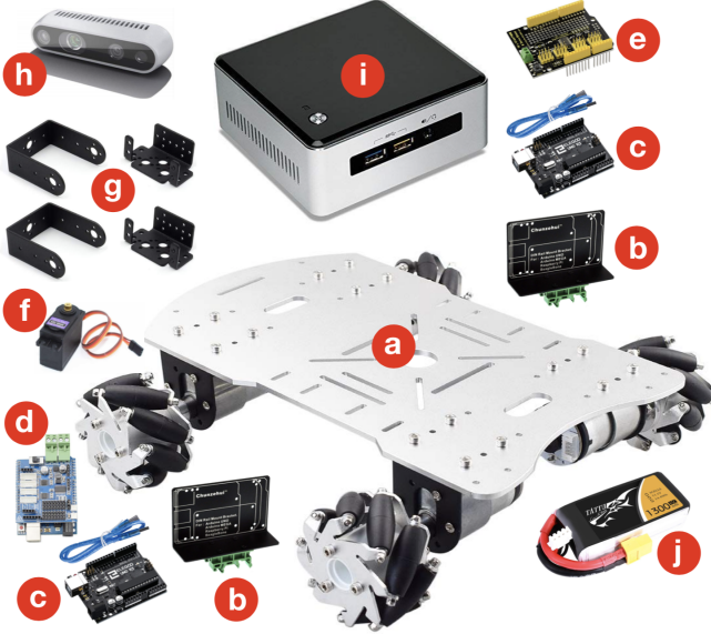
Fig. 2. Various hardware components for the mobile robot. All hardware and electronic designs were performed in-house at Rutgers University by the co-authors of the present paper.
