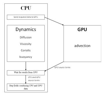
Figure 2. Hybrid dynamics structure
