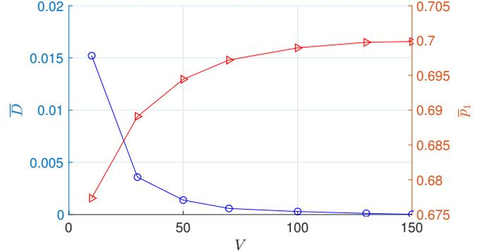
(c) Trade-off between packet drop rate and average power consumption of user 1 for different values of  $V$ .
