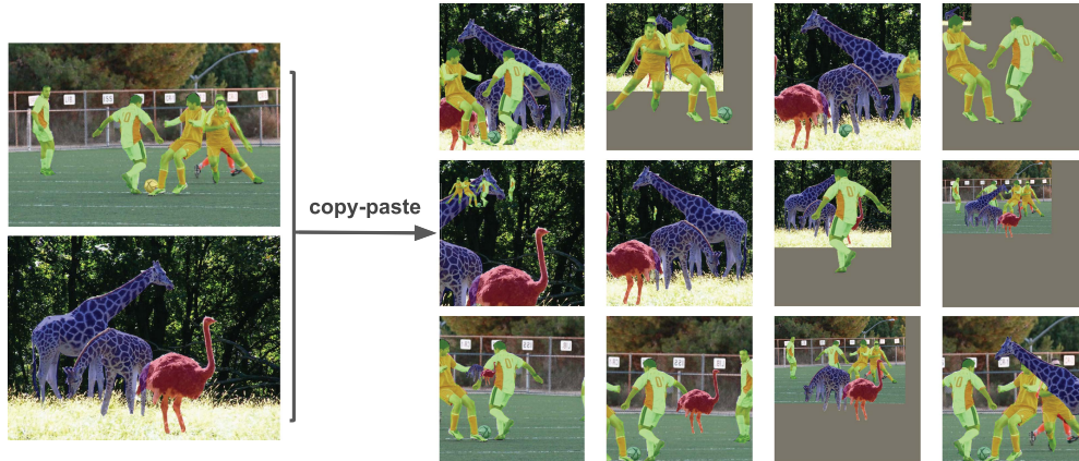
Figure 2. We use a simple copy and paste method to create new images for training instance segmentation models. We apply random scale jittering on two random training images and then randomly select a subset of instances from one image to paste onto the other image.
