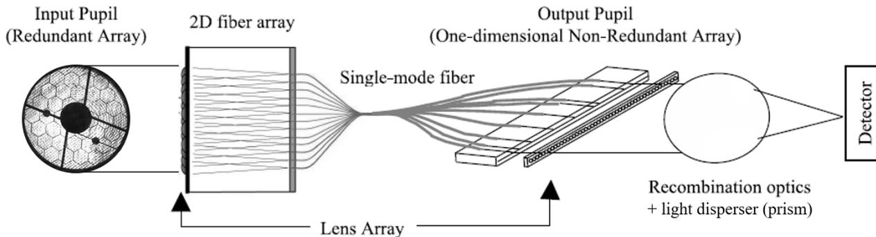
Figure 1. Schematic diagram<sup>9</sup> showing the principle of the FIRST instrument at the Subaru Telescope. The pupil of the Subaru Telescope is divided into several single-mode fibers thanks to a 2D micro-lens array. Light from the different fibers are then set into a one-dimensional non-redundant array, recombined and spectrally dispersed.
