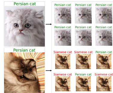
Figure 1: Random noise transformations may lead to a different number of label prediction changes for different images. Here we apply six different transformations sampled from N(0, 0.16^2) .
