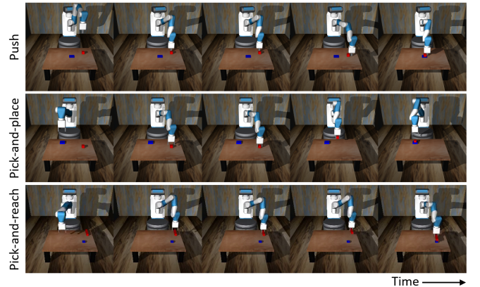
Fig. 3. Top: Example of a pushing expert demonstration. The robot first pushes the red cube forward to align it with the blue target, and then moves to the side to push it sideways onto the target. Middle: Example of pick-and-place expert demonstration. The robot first moves toward the red cube to pick it up, and then moves to the blue target to drop the cube. Bottom: Example of a pick-and-reach expert demonstration. The robot first moves towards the red stick to pick it up at one end, and then reaches the blue target with the other end.
