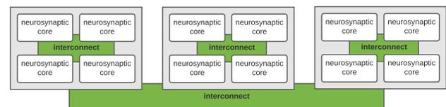
**Figure 1.** Hardware architecture of neuromorphic systems.
