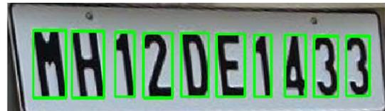
Fig. 7: Letter Detection using WpodNet
