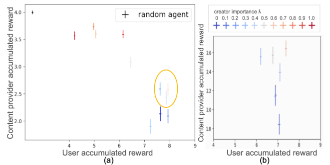
Figure 7: Tradeoff between users and content providers accumulated reward. (a) A properly tuned content provider aware EcoAgent can have a good balance between user utility and content provider utility. (b) In a setup where there exist two identical groups of providers, differing only in initial satisfaction, as expected, there is no tradeoff—we can increase provider utility without sacrificing user utility.
