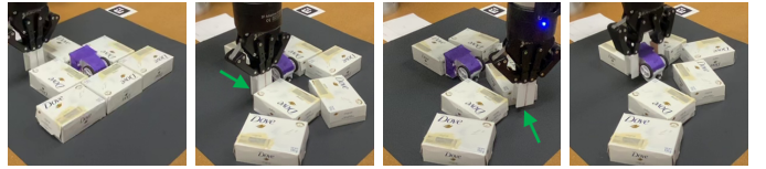
Fig. 8: Test scenario with soap boxes and masked 3D printed vehicle. Two push actions and one grasp action.
