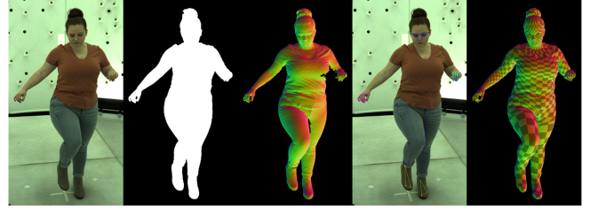
Fig. 7. Data Processing Pipeline. From left to right: input image, foreground body mask, reconstructed 3d shape, detected keypoints, registered surface mesh.
