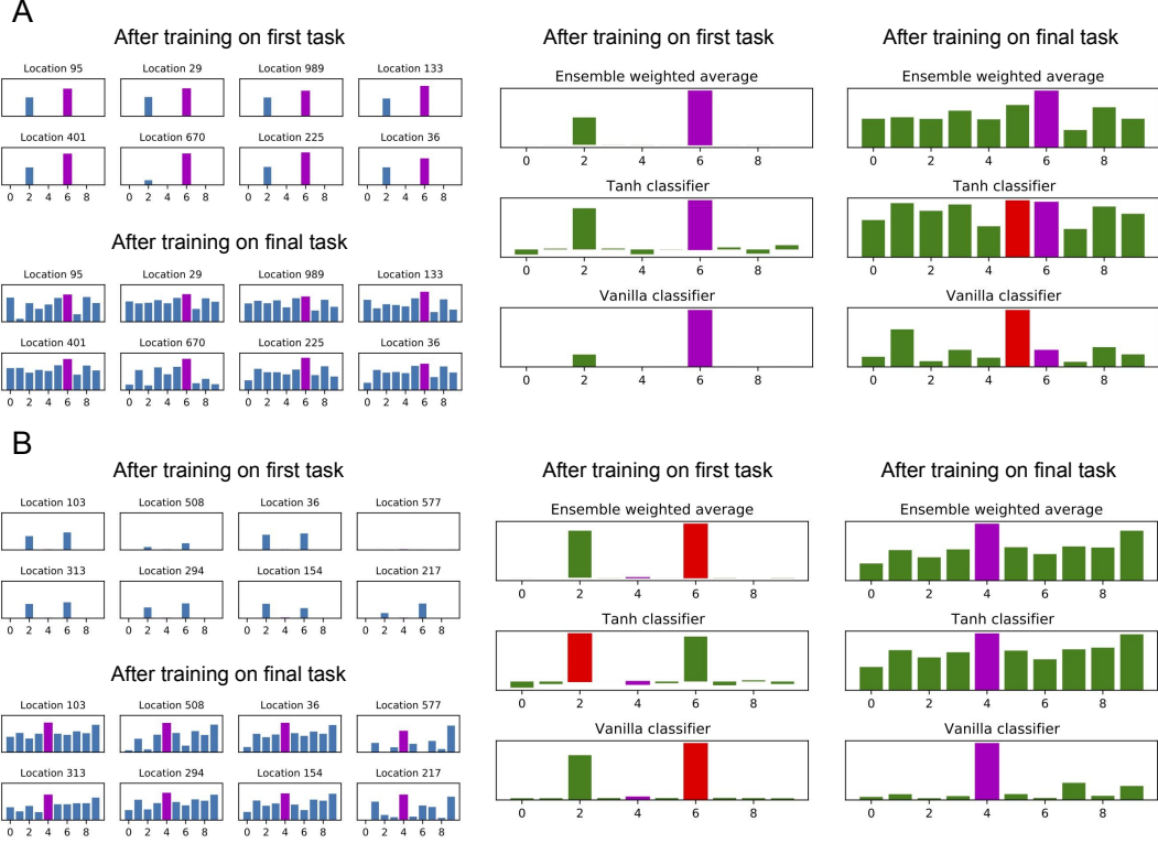
Figure 4: Visualisation of a representative training run for 5-way split MNIST (low data regime). Final layer activations are shown for two sample digits at different points in training. Magenta denotes the correct digit. Red denotes the maximal activation where different from the correct digit. (A): The sample digit (8) belongs to the first task. (B): The sample digit (3) belongs to the final task.
