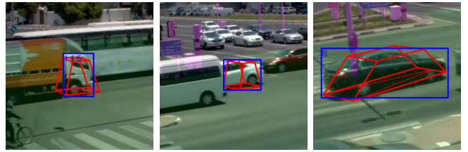
Fig. 7. The dominant cases when UTS yields erroneous 3D tracking results are detection errors especially with large vehicles as trucks and buses (left), dynamic occlusions caused by other vehicles (middle) or orientation initialization errors (right).
