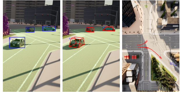
Fig. 1. The left image shows the output of the detector (axis aligned 2D bounding boxes). The reconstructed and tracked 3D bounding boxes are depicted in the image in the middle. The area masked in green color in the first two images is the detection and tracking area that defines where our system should actively operate. The right image shows the same 3D bounding boxes and the center trajectories from a bird's eye view. Images are generated using CARLA Simulator [4]. Best viewed in color.
