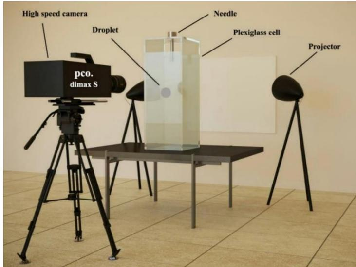
Fig. 1. Schematic sketch of the experimental setup.
