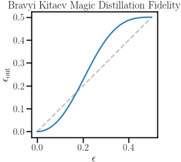
FIG. 1: The output fidelity as a function of input fidelity. The cross over point is \epsilon^* \approx 0.173 . If the input states are not sufficiently close to a T state, then they will limit to the maximally mixed state.
