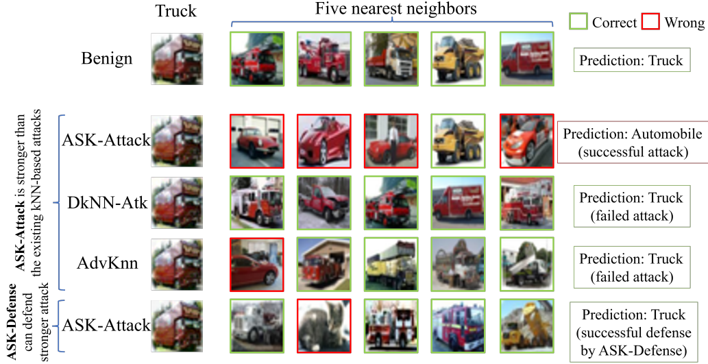
FIGURE 2. Representative example showing superiority of proposed ASK attack (ASK-Atk) and ASK defense (ASK-Def) as compared to previous attack strategies (DkNN-Atk and Adv-Knn). When the DkNN/VGG16 predictor is trained with standard adversarial training [15] on CIFAR-10, for equal perturbation \epsilon , ASK-Atk (2nd row) is more successful than other attacks (3rd and 4th row). Ask-Atk maximizes the proposed ASK loss, and its perturbation of the truck image (top left) flips the classes of 4 out of 5 of the image's nearest neighbors. When DkNN/VGG16 is trained with Ask-Def, which minimizes the maximum ASK loss, it successfully defends against all 3 attacks. In particular, the ASK-Atk can only flip the class of a single nearest neighbor (5th row).
