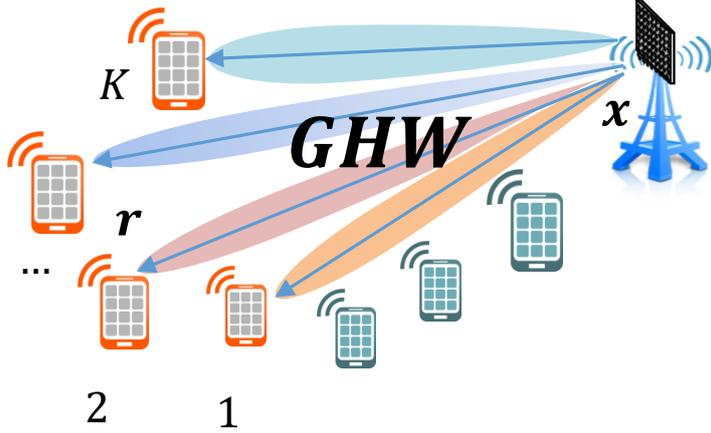
**Figure 1.** An example of the MIMO precoding usage. The problem is to find an optimal precoding matrix  $\mathbf{W}$  of the system given the target Spectral Efficiency (SE) function with the given constraints (24).
