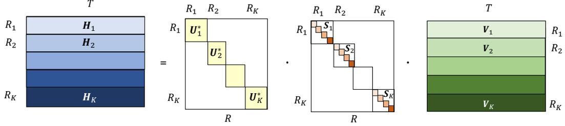
**Figure 3.** The main decomposition of the channel matrix.
