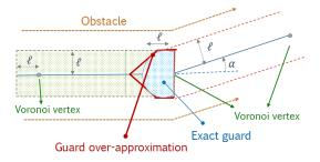
Fig. 6. Over-approximation of guard. l is the look ahead distance of the car. The original exact guard is circular and we linearize it as a convex polytope that is defined using linear constraints.
