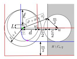
Fig. 5. Consistency of local and global Voronoi diagrams. The blue curve is the global Voronoi diagram. The green dot is lidar, and the pink dot is the waypoint. The gray area is  $H \setminus C_{u,\frac{m}{2}}$ .
