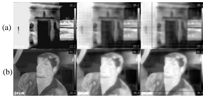
Fig. 3: A comparison of different images showing their RoF. (a) and (b) are images obtained via the FLIR E60 and (c), (d) and (e) are obtained via Sonel KT400 and have different image resolutions. The leftmost images are thermal inputs, the middle ones are Histogram Equalized masked outputs and the right most images are the outputs obtained after running the RoF algorithm on the images in the middle.
