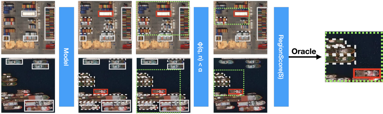
Figure 2: Conceptual illustration of our proposed method, Region-level Active detector Learning (ReAL). A set of partially labeled images ( X_P ) are passed through an object detection model which produces candidate object bounding boxes. A query object is selected around which a context window is dynamically constructed (Eq. 2). Other candidate objects within the context window are filtered by similarity to the query. Regions are then scored by Eq. 3, the highest scoring of which are sent to the oracle for labeling.
