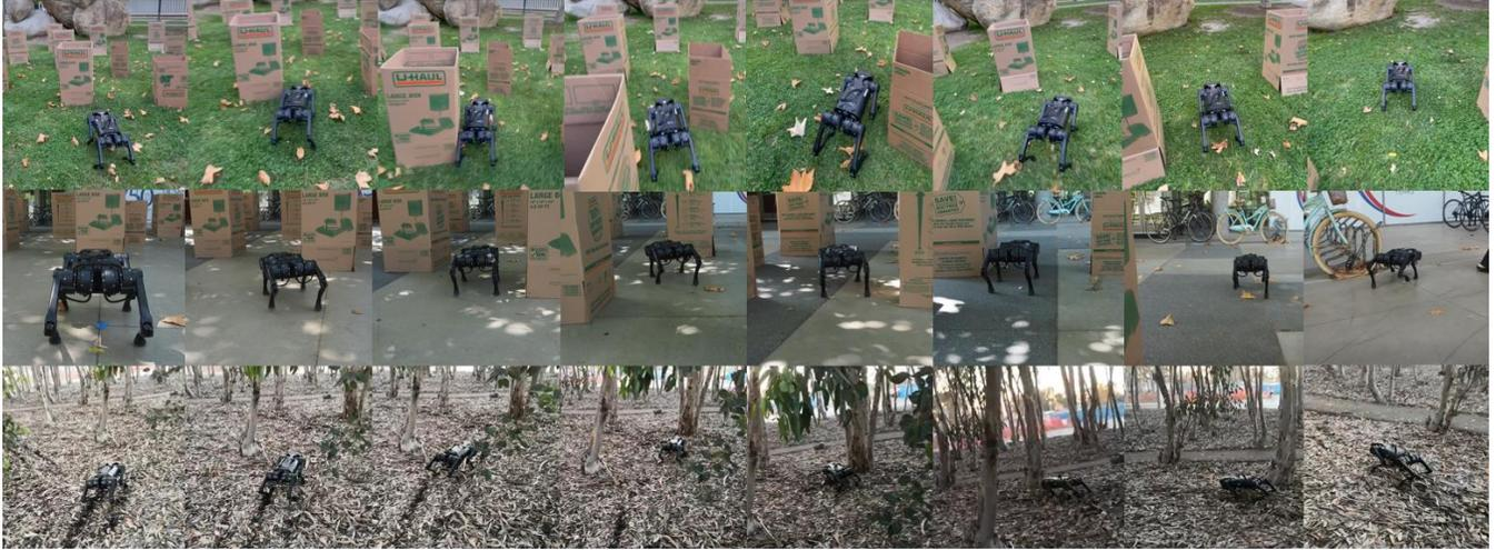
Fig. 1. Our method enables quadrupedal robots to traverse complex environments with obstacles of different shapes in the wild. The learned locomotion policy obtains different agile locomotion skills like flexibly turning before barriers and stably walking on steep lawn, using reinforcement learning. The policy is trained in simulation with our multi-modal delay randomization and deployed in the real-world, unseen scenarios without any adaptation or fine-tuning.
