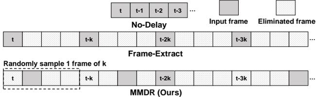
Fig. 5. Comparison of Our Method and Two Baselines. Our method randomly select one frame in each consecutive  $k$  frames, while both baselines use the latest image in a fixed interval (1 for No-Delay and  $k$  for Frame-Extract).
