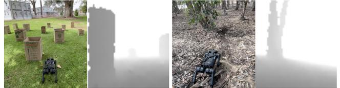
(b) *Real Environments*. We evaluate the generalization ability of policies in real-world scenarios with obstacles of different shapes and sizes on a complex terrain. Due to the noisy reading of the depth camera, some depth values are missing in the depth map, which breaks the shape of an object in the visual observation.
