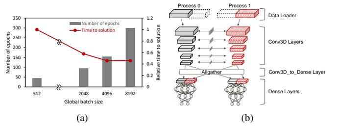
Fig. 4. (a) The number of epochs to solution (left y-axis) in open division for CosmoFlow (see  $\star$ ABCI-2048,  $\star$ Fugaku-16384 in Figure 2b) and extrapolated time to solution (right y-axis, relative to 512 CPUs) as a function of global batch size on Fugaku with data parallelism (local batch size is one). (b) Spatial partitioning (2x1) for model-parallelism in CosmoFlow.
