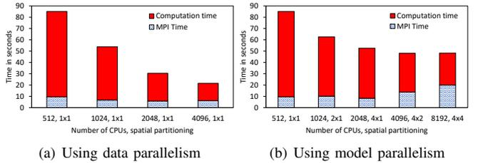
Fig. 5. Elapsed time for the first two epochs of CosmoFlow on Fugaku using data-parallel scaling (local batch size one, no spatial partitioning) and (hybrid) model-parallel scaling (global batch size 512, with spatial partitioning) starting from a data-parallel baseline with 512 CPUs. Time spent in communication (MPI) is measured as in section V.
