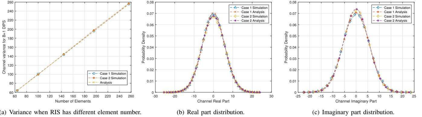
Fig. 3: The variance, real part distribution and imaginary part distribution of the channel assisted by  $B = 1$  DIPS RIS.
