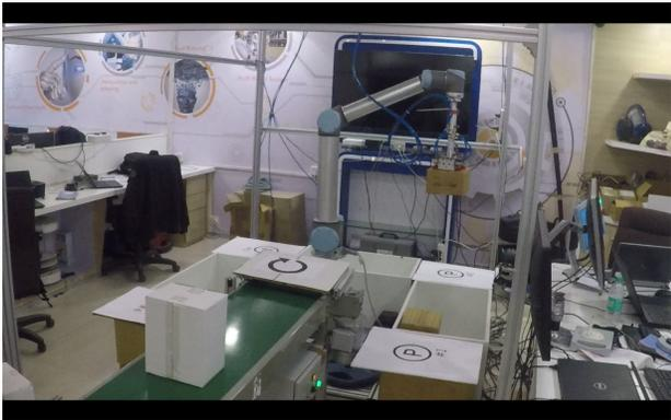
Fig. 1: Lab mock-up of robotic arm packing boxes into bins.
