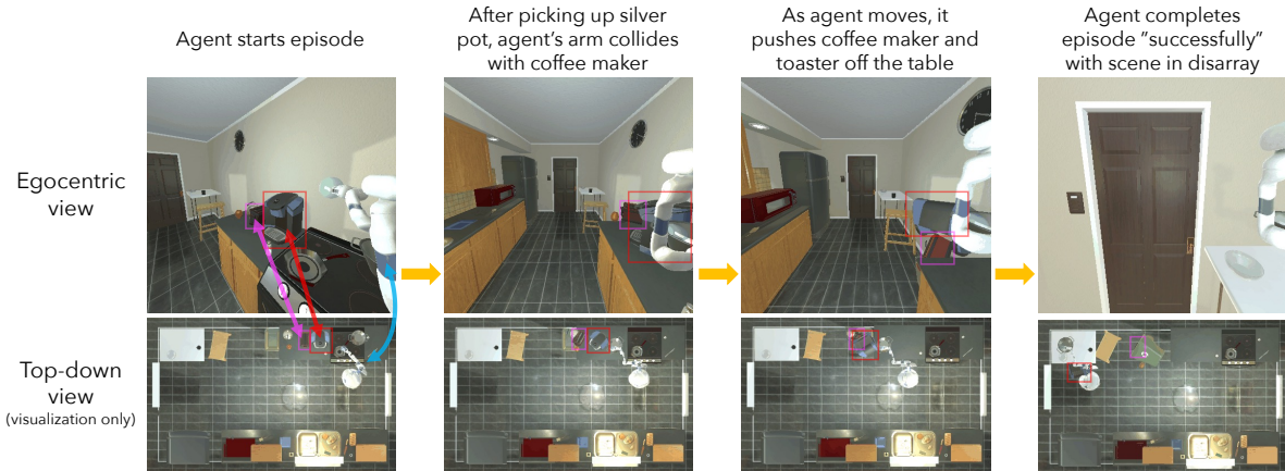
Figure 1. Success with disturbance. A robotic ManipulaTHOR [16] agent attempts to complete an ArmPointNav task where it must pick up and move one object from one side of a kitchen to another. A well-trained agent (in white) successfully moves the target object (a silver pot) from a source location (stove burner) to a target location (dining table). Despite this success, the agent disturbs several objects (including a coffee maker and a toaster) when moving its arm and body. Both the coffee maker and toaster are pushed off the countertop and the coffee maker is further pushed across the kitchen, a catastrophic outcome in the real world. The figures show both RGB egocentric and top-down views, while the agent only has access to egocentric observations.
