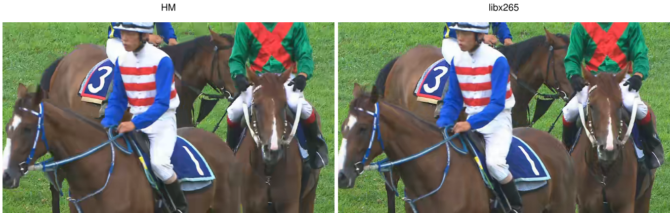
Figure 8. Codec Comparison. HM reference encoder vs. libx265 at QP37. While the artifacts produced by the different encoders are different, the overall perceptual quality is similar. This is likely because of CQP encoding which does not leave many options for the encoder to make intelligent rate-distortion decisions.
