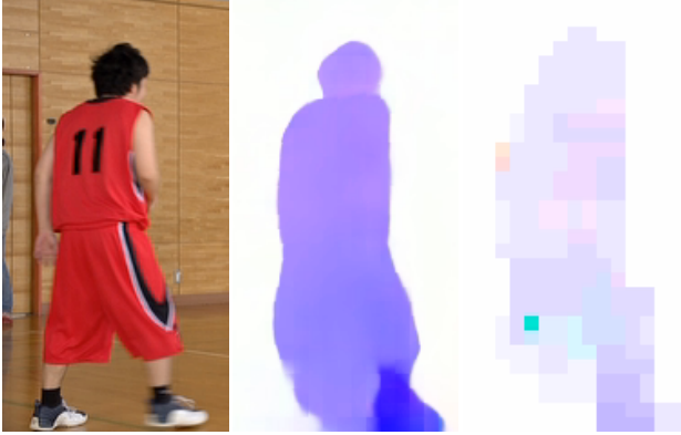
Figure 2. Motion Vectors. Motion vectors resemble downsampled optical flow. Left: reference image. Middle: optical flow. Right: motion vectors extracted from the video bitstream. Optical flow was computed with RAFT [11].
