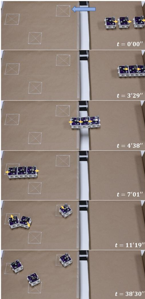
Fig. 9: These video frame sequences show that three initially separated robots are able to couple with each other, go cross a gap (60 mm), decouple, and go to their individual goal locations (white squares). In the first frame, the robots start on platform on the right. They will need to cross the gap and reach the left platform. The blue arrow shows their goal direction, and yellow arrows show their current direction of motion of each robot.
