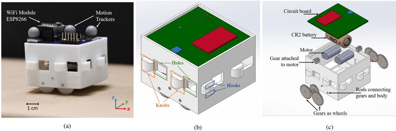
Fig. 2: (a) A PuzzleBot with motion trackers in Vicon system. The  $xyz$  axis of the robot body frame points front, left, and up, correspondingly. (b) Design of the assembled robot. Each side of the robot body consists of two knobs and holes. There are hooks on top and bottom of each knob. (c) An exploded view of the PuzzleBot with mechanical and electrical parts.
