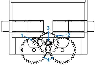
Fig. 5: Side view of the robot with double reduction gear. The first pair consists of gear  $g_1$  and gear  $g_2$  where gear  $g_1$  is attached to the motor and  $g_2$  is on the center rod. The second part of the double reduction gear consists of  $g_3$  and  $g_4$ , where  $g_3$  is attached to  $g_2$ . The two identical side gears are both referred to as  $g_4$ . The two  $g_4$  also serve as wheels.
