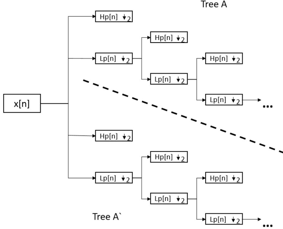
Figure 3: The structure of three scale level of DTCWT.
