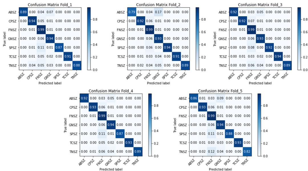
Figure 8: Confusion matrix for 7-class classification problem having 5-fold cross-validation: 1st to 5th fold (Left to right, top to bottom).
