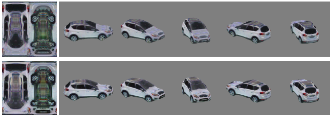
Fig. 4: 3D reconstruction outputs of models trained with unpruned and pruned datasets. First column shows texture map predictions, other columns show the rendering results from different viewpoints. First row, mesh learning results from the multi-view dataset. Second row, mesh learning results after removing the frames with wrong camera estimation. Notice the improvements on the headlight and plate after pruning the dataset.
