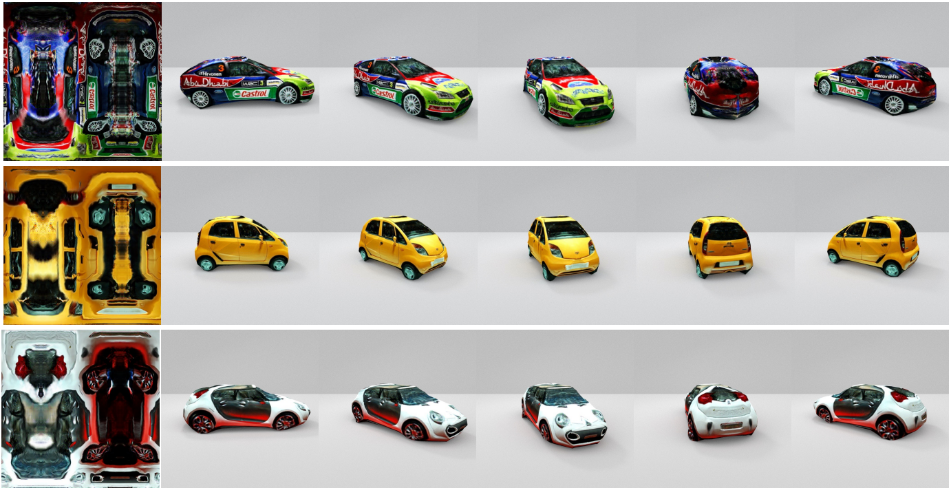
Fig. 1: Given a multi-view image sequence with no annotations, we infer high quality textured 3D models by utilizing pre-trained networks. The 3D model is presented as triangular mesh and a texture map which can then be used to render novel views. The texture maps are learned with a novel GAN architecture and present fine details that make textured 3D models look highly realistic.
