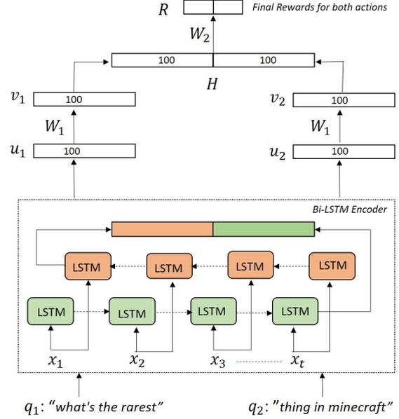
Figure 2: The Bi-LSTM Siamese DQN network for calculating rewards for both WAIT and SEARCH actions. The numbers represent the dimension of outputs generated by each layer.
