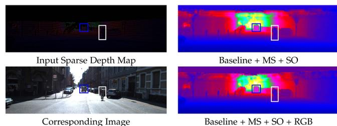
Fig. 4. Qualitative comparison of unguided and RGB guided depth completion where MS and SO denote multi-scale structure and sparsity-invariant operations, respectively. From [48].
