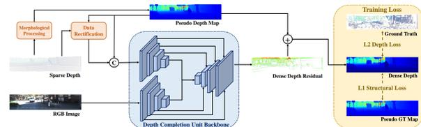
Fig. 9. The pipeline of the DenseLiDAR where depth completion is decomposed as learning of a coarse depth map and a residual depth map. From [34].
