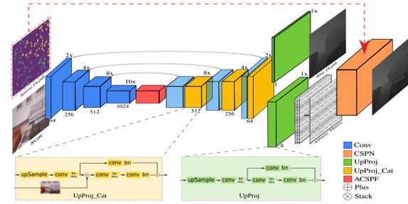
Fig. 10. The framework of CSPN based depth completion. The CSPN module is plugged into the network to rectify a coarsely predicted depth map. From [111].
