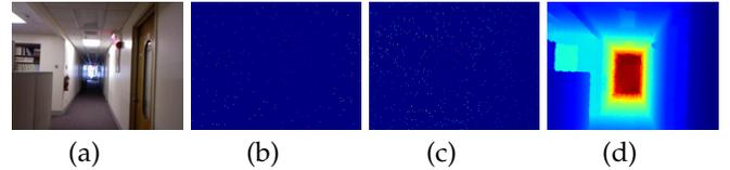
Fig. 14. A sample image from the NYU-v2 dataset [99]. (a) An RGB image. (b) A sparse depth map (200 points). (c) A sparse depth map (500 points). (d) The corresponding ground truth depth map.
