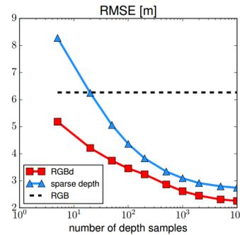
Fig. 3. The RMSE for unguided and RGB guided depth completion on the KITTI dataset. From [77].
