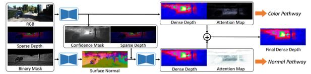
Fig. 8. The pipeline of the DeepLIDAR where surface normal is used as an intermediate representation of a depth map. From [88].
