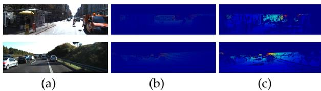
Fig. 13. Sample images from the KITTI depth completion dataset [109]. (a) RGB images. (b) Raw sparse depth maps. (c) Ground truth depth maps.
