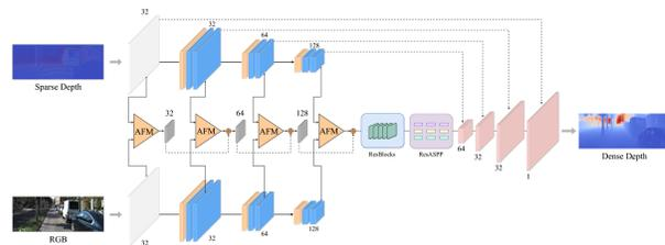
Fig. 5. The diagram of the multi-scale adaptation fusion network (MAFN). The framework is a dual-encoder network where features extracted from the RGB encoder and the depth encoder are fused with the adaption fusion (AFM) module at multi-scales. From [137].
