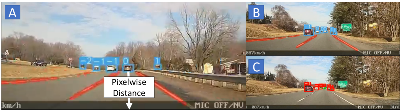
Fig. 3. The methodology to calculate the pixelwise distance from the lead vehicle. (A) detection the lead vehicle using a combination of lane tracking and object detection. Enhancing the high number of false positives in detection as the lead vehicle (B) through post-processing (C)
