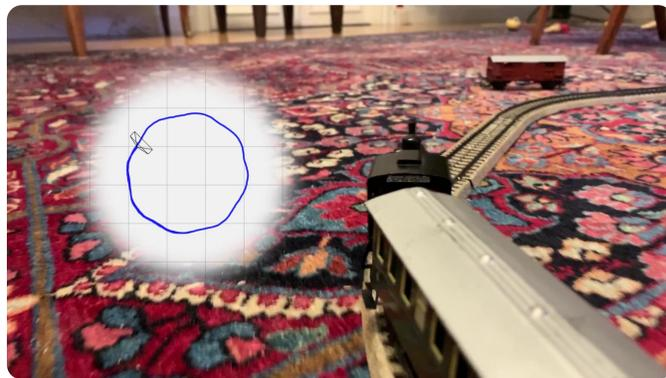
Fig. 1. Motivating example: A visual-inertial odometry setting with a smartphone camera attached to a model train car. The high-frequency jitter from the tracks and severe motion blur degrade both the IMU and camera data, which calls for principled inference methods. The overlaid track shows that the estimates do not drift away (grid 50 cm).
