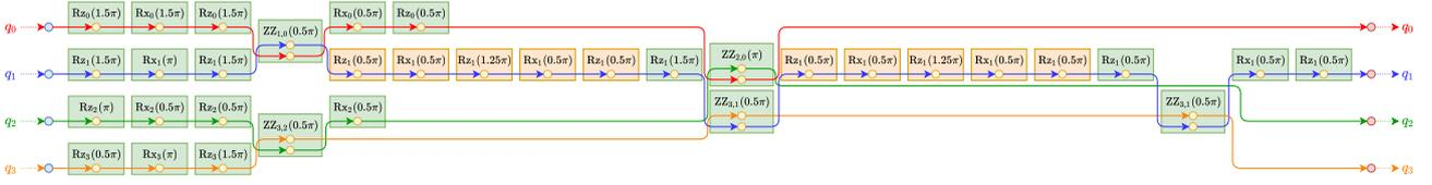
(a) Example from Fig. 8c after applying the transformation of single-qubit gates into our trapped-ion native gate set. The two  $R_{X1}(0.25\pi)$  gates in Fig. 8c are transformed into the two orange gate sequences, and their angles are included in the phase of the  $R_{Z1}(1.25\pi)$  gates. All single-qubit gates of the circuit are in our trapped-ion native gate set  $\mathcal{N}$ .
