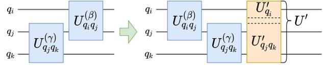
Fig. 15: The two superblocks represented by the unitaries  $U_{q_iq_j}^{(\beta)}$  and  $U_{q_jq_k}^{(\gamma)}$  are commuted. Since in general it is not guaranteed that both unitaries are commutable, a correction unitary  $U'$  is inserted, which corrects the error introduced by the commutation of the superblocks. Under certain conditions  $U'$  can be factorized into two correction unitaries  $U'_{q_i}$  and  $U'_{q_jq_k}$ .
