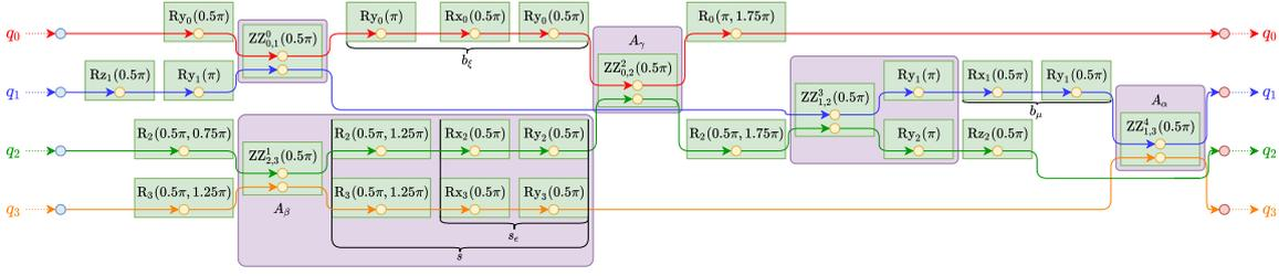
(a) The same gate sequences  $b_\mu$  and  $s_e$  are executed on  $q_1$  and  $q_3$  before the block  $A_\alpha$ . On  $q_1$  the gate sequence  $b_\mu$  is a blockless sequence, while on  $q_3$  the gate sequence  $s_e$  belongs to a different block  $A_\beta$ . To eliminate the blockless sequence  $b_\mu$ ,  $b_\nu$  and the gates on  $q_3$  from  $s_e$  can be added as a predecessor sequence to  $A_\alpha$ .
