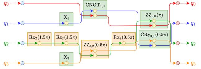
Fig. 6: Example from Fig. 5c with the macro matching applied. Since only the gate  $\text{CRy}_{3,2}(\pi)$  of the CRy gates in Fig. 5c satisfies the condition  $\theta = \ell\pi$  with  $\ell \in \mathbb{Z}$ , only this gate is replaced by the orange gates.
