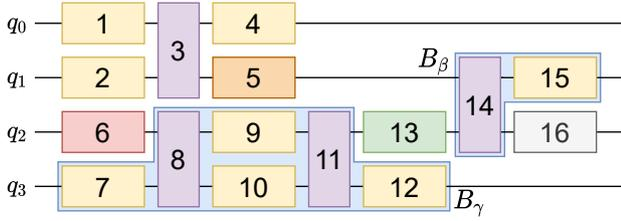
(a) Example from Fig. 13b with the superblocks  $B_\beta$  and  $B_\gamma$ . The non-yellow blockless sequences can be added completely, partially or not to the adjacent superblocks. Since no gates are allowed on the common qubit  $q_2$  between the two superblocks, blockless sequence 13 must be added completely to  $B_\beta$  or  $B_\gamma$  or divided between them.
