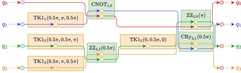
(b) Example from Fig. 6 after applying Pytket's SquashTK1 pass as described in Sec. 4.4. Again, all sequences of single-qubit gates have been replaced by exactly one orange TK1 gate. In contrast to the CliffordSimp pass, the green two-qubit gates remain unchanged.
