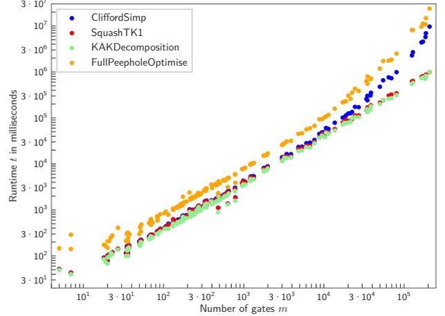
(b) Runtimes of our compiler when executed without the block commutation with correction unitaries. In this case, the `CliffordSimp` and `FullPeepholeOptimise` approaches lead to a nonlinear scaling of the runtimes, while the `SquashTK1` and `KAKDecomposition` approaches behave linearly with the number of gates.
