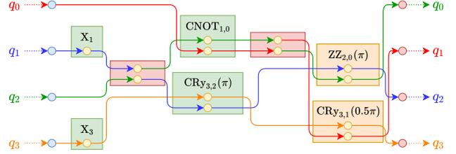
(b) The SWAP gate elimination is also applied to the second SWAP gate (the right red box). Consequently, the outgoing edges are exchanged compared to (a). This means that after the SWAP gate,  $q_0$  follows the green path and  $q_1$  the red one.
