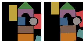
Fig. 4: Examples of using the grasp classifier to produce probabilities to grasp the object at center (blue in this case). Here we used an RGB image for illustration purpose (input should be a depth image).
