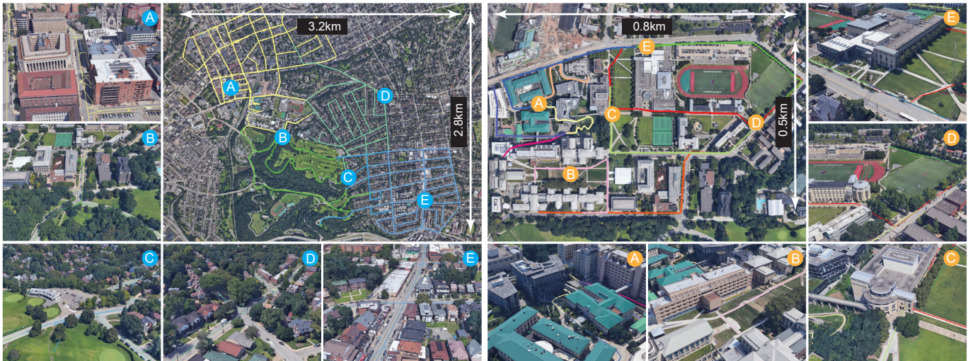
Fig. 7. Self-collected Datasets. Both Pittsburgh and Campus datasets are collected with our data-collection device (Velodyne-16 and Xsens MTI-300 IMU). The Pittsburgh dataset includes 4 zones (colored in yellow, green, cyan, and blue), which covers street blocks, residential areas, parks and commercial buildings. The Campus dataset is shown in the pictures on the right, which covers the main campus area of Carnegie Mellon University.
