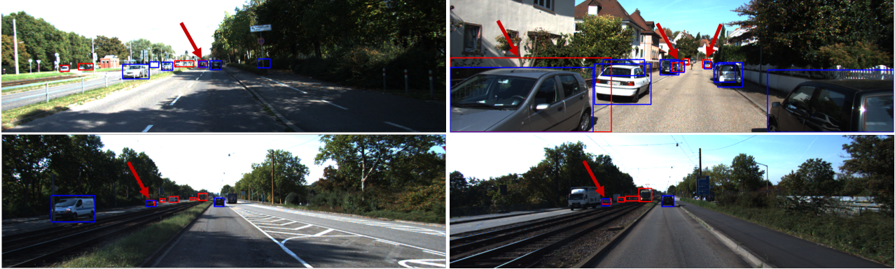
Figure 7. Comparison of the ground truth and pseudo-labels. We show the ‘DontCare’ cases in the ground truths in red, and the pseudo-labels in blue. These cases suggest the proposed method can provide more effective supervision than ground truth in some cases. We only show the 2D bounding boxes for clearer presentation.
