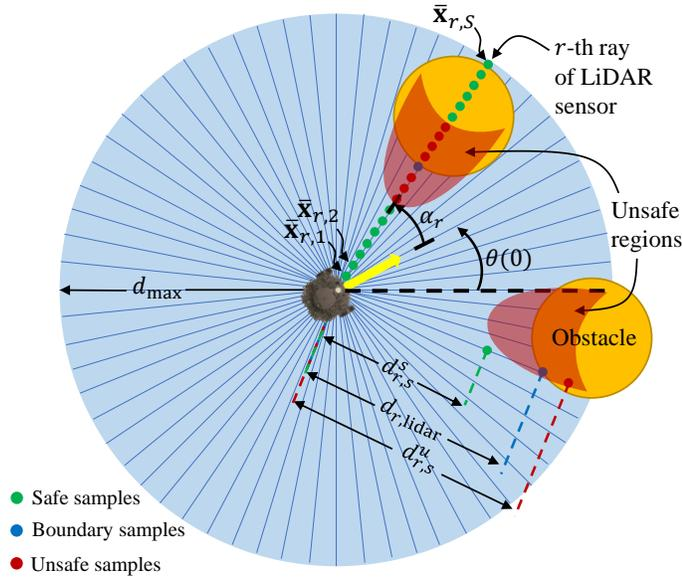
Figure 1. LiDAR sensor rays and point sampling in safe and unsafe regions within the sensing range of the LiDAR. The unsafe samples are taken from the red shaded regions and the safe samples are in areas excluding the unsafe regions.  $d_{r,s}^s$ ,  $d_{r,lidar}$ ,  $d_{r,s}^u$  show the distances of the robot to the safe, boundary, and unsafe samples on a ray of LiDAR.
