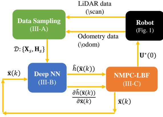
Figure 3. Block diagram of the NMPC-LBF method described in Eq. (11). `\scan` and `\odom` are ROS topics through which the states of the robot and the LiDAR measurements would be available.
