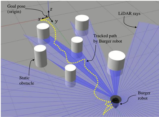
Figure 4. A snapshot of the simulation of scenario 1 in Gazebo. The robot should stabilize to the goal position at the origin of the global frame.
