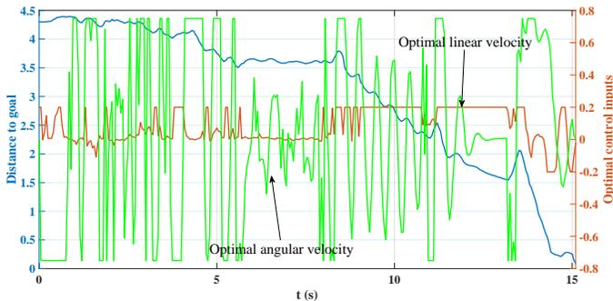
Figure 5. Distance to goal position and optimal control inputs over time of the robot in scenario 1.
