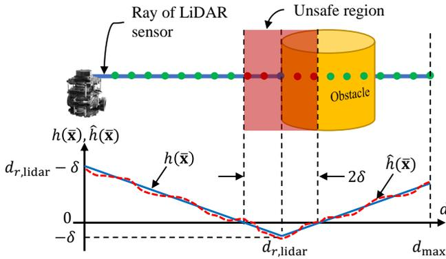
Figure 2. An illustration of ground-truth BF,  $h(\bar{\mathbf{x}})$ , and approximation of BF by the DeepNN,  $\hat{h}(\bar{\mathbf{x}})$ , on a single ray of LiDAR along with a 2D visualization of safe and unsafe samples and a sample on the boundary of an obstacle. We note that the sample points are defined in the  $x-y$  plane with a height of zero.
