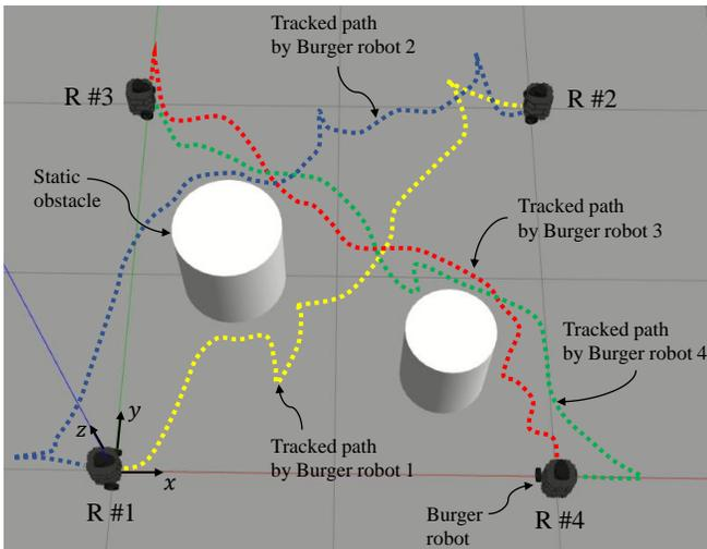
Figure 6. A snapshot of the simulation of scenario 2 in Gazebo. All robots should stabilize to their goal positions while avoiding collisions with other robots and static obstacles.
