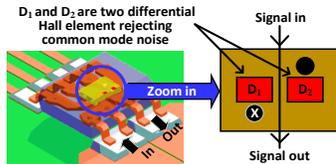
Figure 4: A basic overview of the differential sensing.
