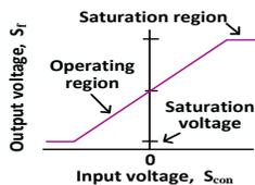
Figure 2: Operating and saturation region of a sensor.
