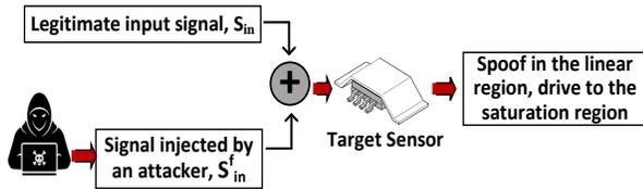
**Figure 3: Basic components of the sensor attack model.**
