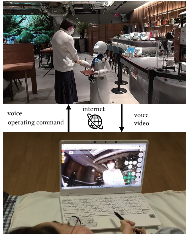
Figure 2: Operation of the avatar robot OriHime-D by a pilot with disabilities at the Avatar robot cafe.
