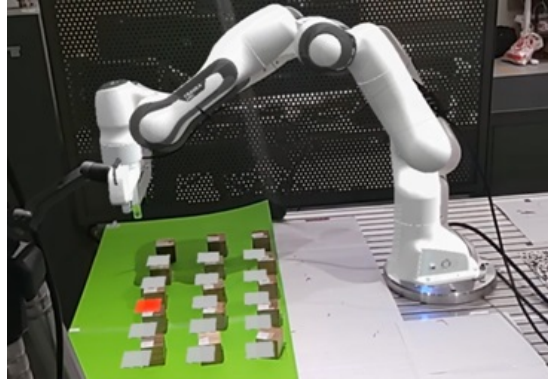
Fig. 1. User's view when collaborating with the robot arm using our AR joint action framework. The block selected by the robot is highlighted in red to convey to the user the robot's intention of picking up the block.
