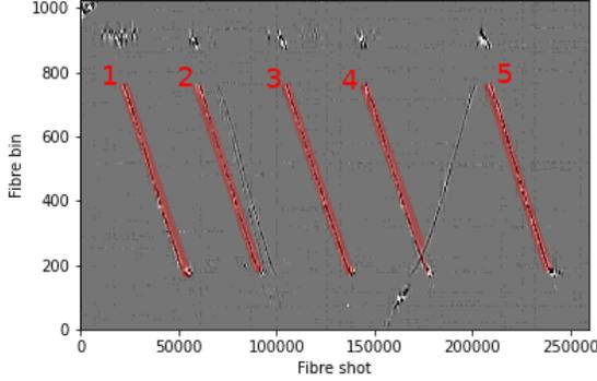
Fig. 2. Section of DAS collected data for 50 km/h experiment showing the five target vehicles in addition to two unwanted ones (taken from AllCars-1p).
