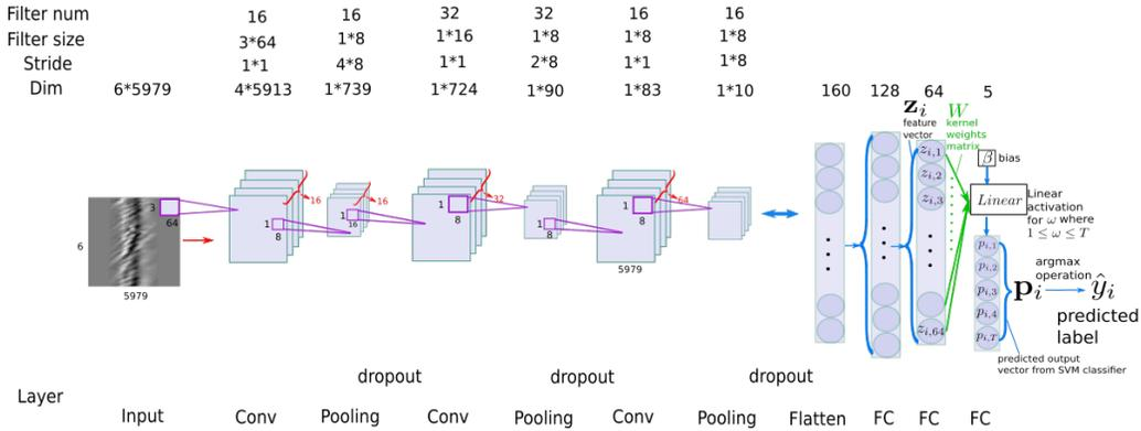
Fig. 4. The 2D-CNN architecture is used for vehicle occupancy detection. It is similar to 1D, however, since the first dimension was small, we limited the width of convolution stride size (set to 1) to preserve more information in the first dimension. The parameters of Flatten, Fully Connected, and Classification layers have the same setting as 1D-CNN.
