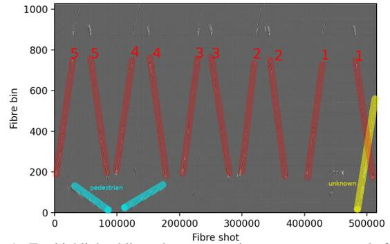
Fig. 1. Ten highlighted lines show car moving at a constant speed of 60 km/h. Each line is labelled with the number of passengers (RC-Mix).
